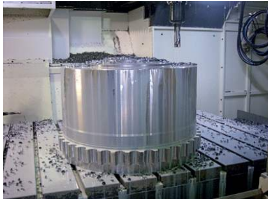
Machining hub TCB®-HD-10200.
