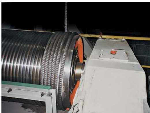
Hoisting mechanism in a steel picking line.
